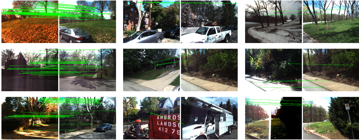
Figure 10. Localization with HF-Net on CMU suburban. For each image pair, the left image is the query and the right image is the retrieved database image with the most inlier matches, as returned by PnP+RANSAC. We show challenging successful queries (left), failed queries due to an incorrect global retrieval (center), and failed queries due to insufficient local matches (right).
