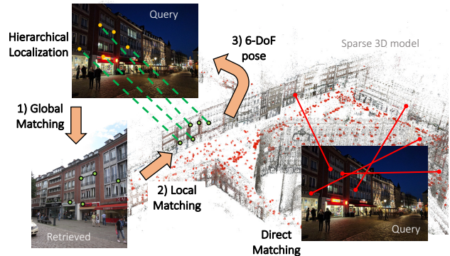
Figure 1. HF-Net working principle. We start by performing global matching, which helps us to remain computationally efficient and improves the robustness in challenging situations. Then, using powerful local features lets us establish reliable correspondences and estimate an accurate 6-DoF pose.
