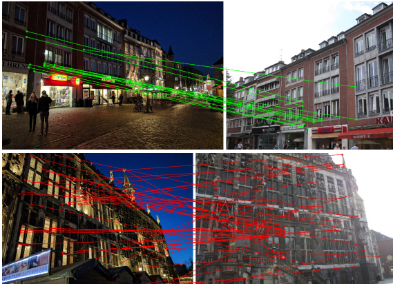
Figure 4. Successful (top) and failed (bottom) HF-Net queries. The top query was successfully retrieved by a HF-Net global descriptor despite the appearance change. Then, it was successfully matched by HF-Net local descriptors. SIFT descriptors failed in this case. The bottom query failed as local matching did not find enough consistent correspondences because of visual aliasing.
