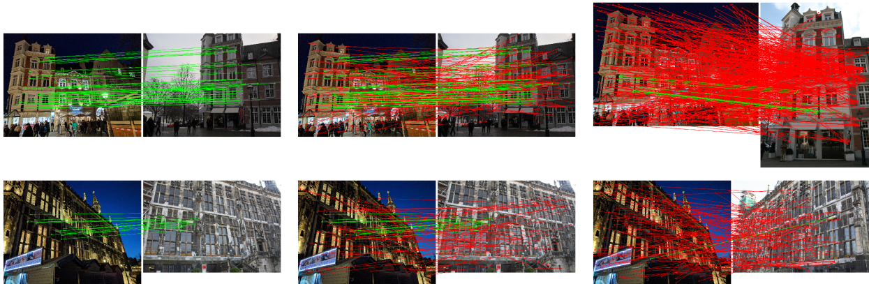
Figure 11. Comparison between HF-Net and NV+SIFT on Aachen night. Each row corresponds to one query for which HF-Net returns the correct location but NV+SIFT fails. We show the matches with one retrieved database image, labeled by PnP+RANSAC as inliers (green) and outliers (red). We show the inliers of HF-Net (left), all the matches of HF-Net (center), and all the matches of NV+SIFT (right). HF-Net generates significantly fewer matches than SIFT, thus reducing the computational footprint of the local matching. At the same time, more of its matches are inliers, increasing the robustness of the localization. The higher inlier ratio reduces the number of required RANSAC iterations.
