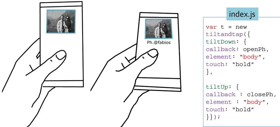
Figure 3.1: Jerk tilting example and its correspondent code using TAT.
