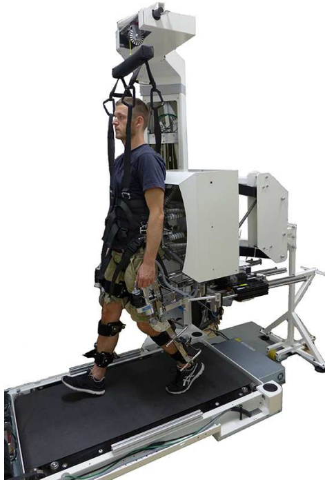
Figure C.1: System overview including frame, treadmill, 2D BWS, MUCDA pelvis module, and actuated orthoses.
