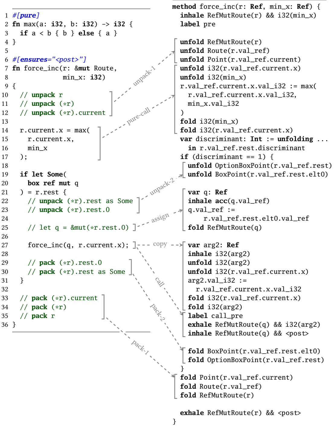
Fig. 8. An encoding of force_inc to Viper. The function is augmented with pack and unpack operations, and is then translated to the Viper method shown on the right. The encoding of the postcondition <post> is in Fig. 10. Note that Rust implicitly dereferences r when accessing its fields.
