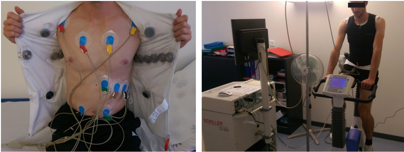
Figure 12: Test setup with both the cooperative-sensor system and the gold-standard medical device (Cardiovit CS-200) connected to the subject (left) and subject performing the exercise stress test (right).
