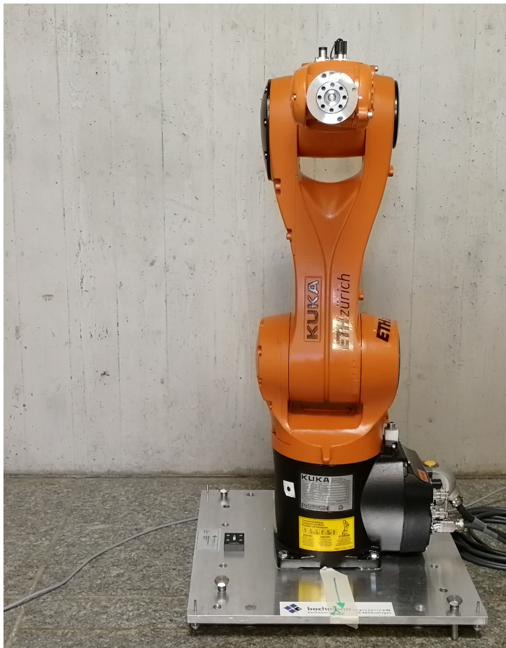
Figure 5.4.2 : Front view of the KUKA Agilus KR 6 R900 sixx. It can easily be seen that all links and joints are in one plane.
