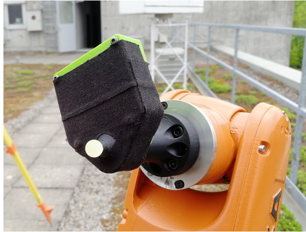
Fig. 6. Illuminated spherical target mounted on the robot. The picture was taken during the offset calibration.
