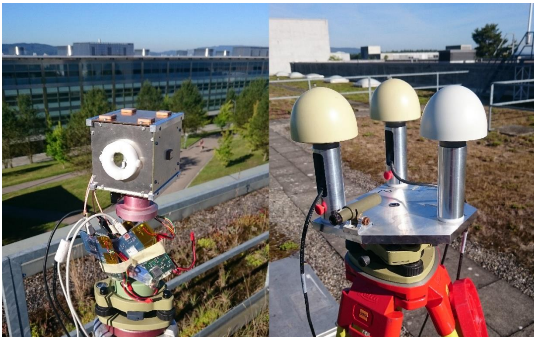
Fig. 2 a) A model of CubETH during measurements for the PCV calibration. Four antennas are located on a common ground plane on the upper face. The side antenna (not used) is visible on the right side. Each antenna is connected to a u-blox GNSS receiver. b) Experimental setup for antenna attitude system calibration. The aluminum plate can be oriented with the help of the telescope. The three antennas of the type Trimble Bullet III can be freely turned and swapped to another location.
