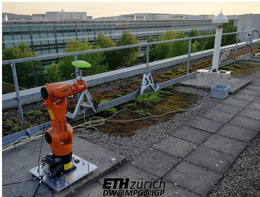
Fig. 5 GNSS antenna calibration set-up. The KUKA robot with a JAVAD GrAnt-G3T antenna (to calibrate) is visible in the foreground on the left. On the right, on the white pillar, the reference antenna of type Septentrio PolaNt Choke Ring B3/E6. The length of the baseline is approximately 5 m.
