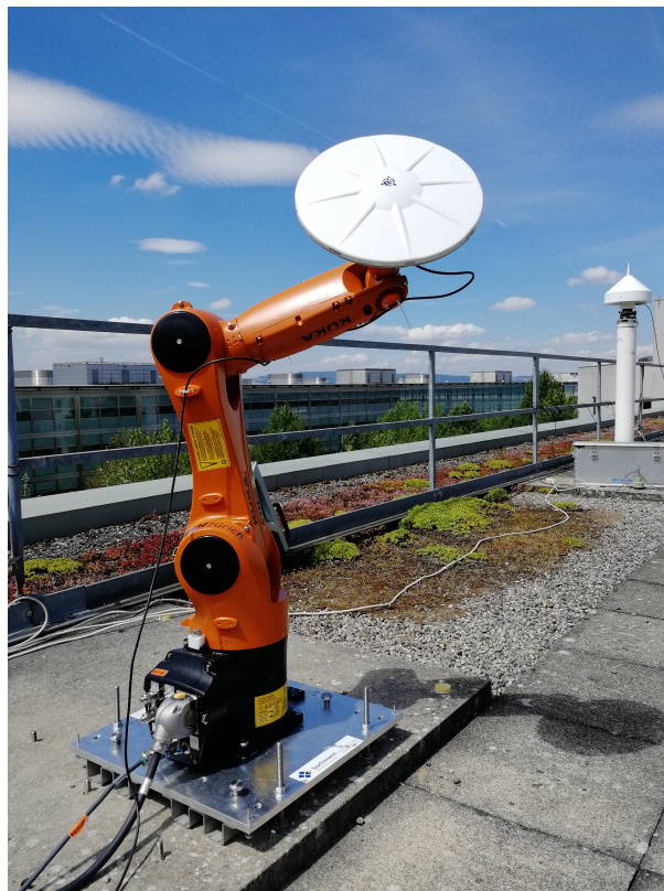
Figure 5.0.1 : KUKA Agilus KR 6 R900 sixx mounted on the roof of the Institute of Geodesy and Photogrammetry (IGP) at ETH Zurich. The robot is performing a GNSS antenna calibration. The aluminium plate serves as interface between the four bolts inserted into the concrete foundation and the robot base. The white antenna in the back is used as reference station.
