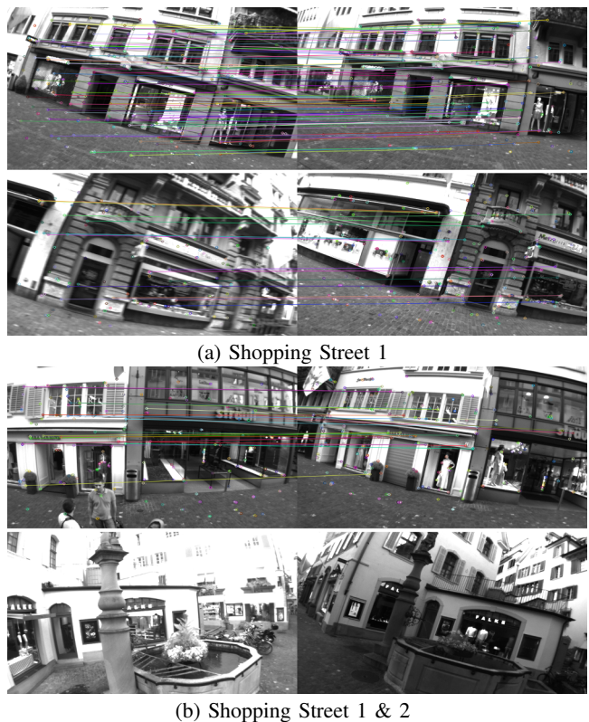
Fig. 4: Example loop-closures from the Shopping Street dataset tested with the proposed approach. The loop-closures in (a) demonstrate robustness of the proposed approach to viewpoint changes and small motion blur (bottom left). In (b), the top image is an example of a loop detected across the Shopping Street 1 and 2 sequences exhibiting big changes in viewpoint and scene appearance, while the bottom image depicts a false negative, where the viewpoint and illumination changes proved too large for a loop-closure match.
