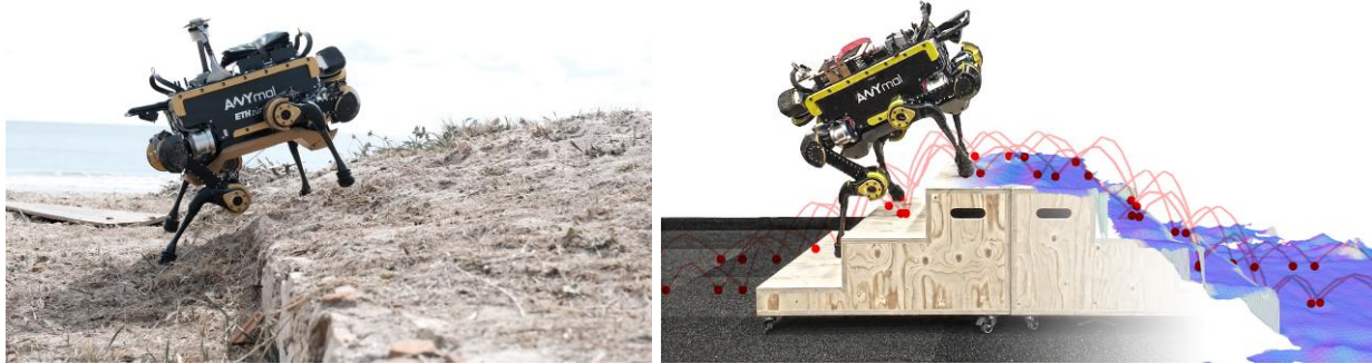
Figure 3: The robot ANYmal walking blindly on a sandy slope at the ERL challenge (left) and climbing a set of stairs (right). Blind walking is based on an optimization-based approach to controlling a dynamic gait, i.e., trotting gait. Climbing over challenging obstacles like stairs includes map-based motion planning. Moreover, footholds (red dots) and base and leg motions (red lines) are generated by processing a terrain map with the help of onboard sensors (Fankhauser et al., 2018a).
