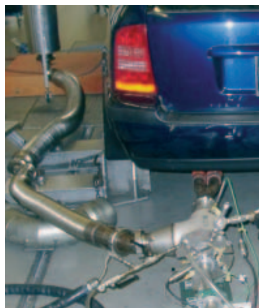
Fig. 2: Set-up of the primary dilution unit attached to the exhaust system of the vehicle.
