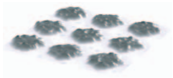
Fig. 2: A simulated microscopic toner profile of a "clustered dot halftone" at nominal 30% area coverage. The illustrated area has a dimension of 1 x 1 mm and is illuminated from the rear right corner.
