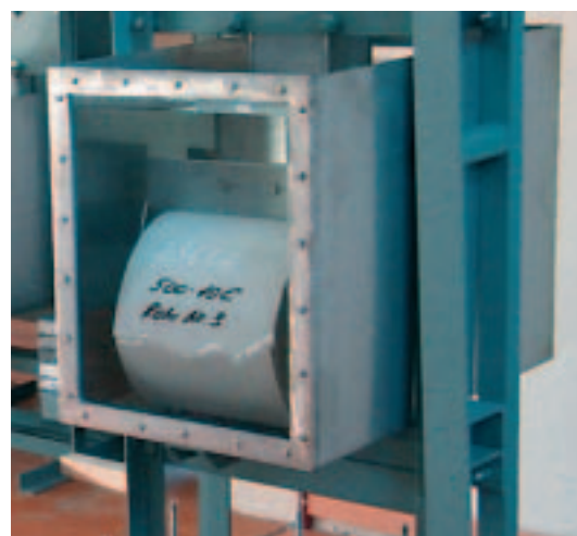
Fig. 1: Testing systems for long-term creep test of pipes in wet condition.
