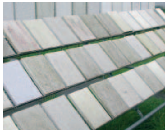
Fig. 2: Outdoor exposition of specimen, coated with different plasters/paints. Different colors indicate different biofilm communities.
