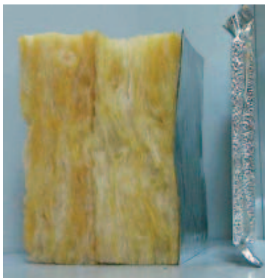
Fig. 1: Conventional mineral wool thermal insulation board and a VIP with equal thermal resistance.
