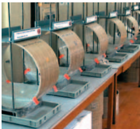
Fig. 3: Testing systems for long-term strain corrosion testing of GRP pipes.
