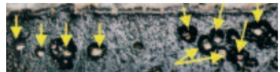
Fig. 3: Formation of bubbles after 2.5 years of weathering. Opposing contact area between joint sealant and concrete edge.
