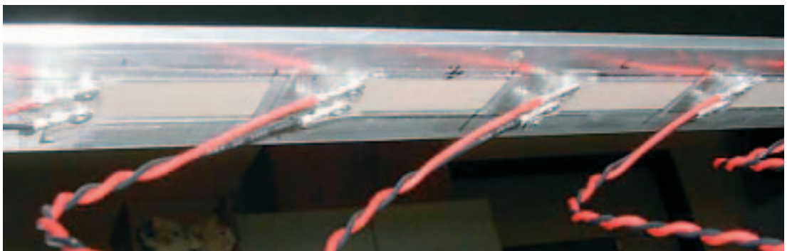
Fig. 2: Prototype of radiation mode sensor (detail).
