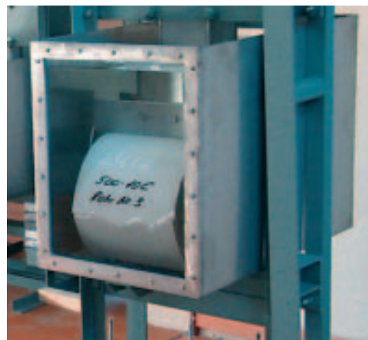
Fig. 1: Testing systems for long-term creep test of pipes in wet condition.
