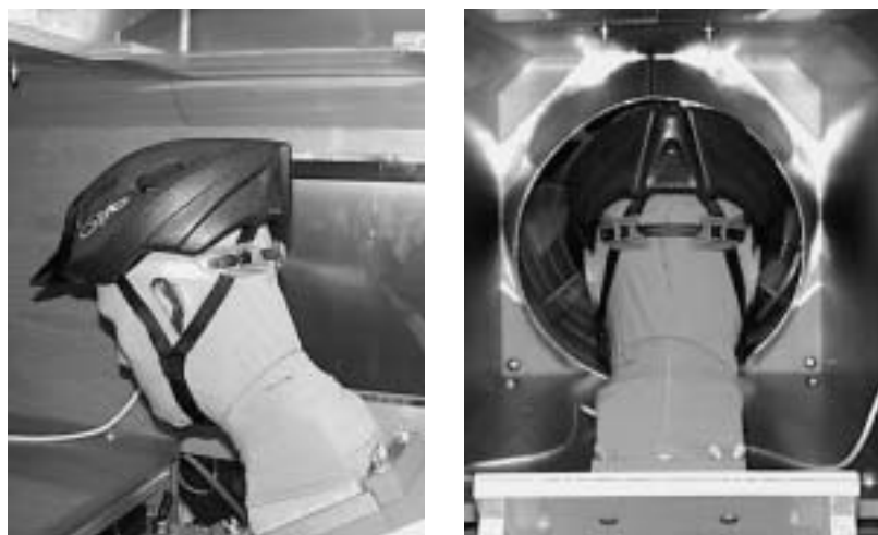
Fig. 1: Apparatus used. The headform is shown at the 30° tilt angle, placed at the mouth of the wind tunnel, all located in a climate chamber.
