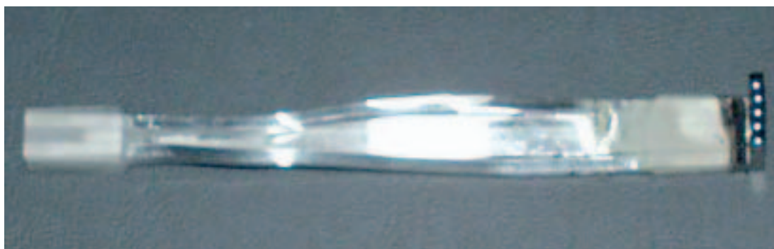
Fig. 3: Package of five imaging fiber bundles, each 1.7 mm square, as used for proof of operation.
