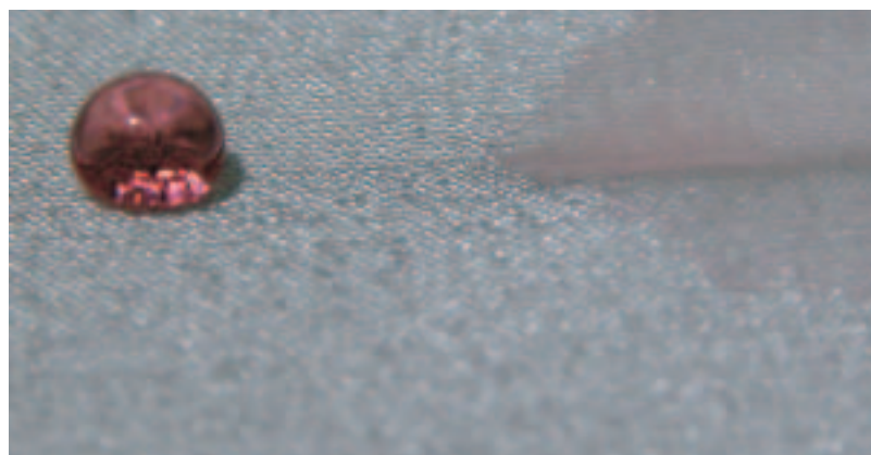
Fig. 4: Drop of colored water on a silk fabric which was rendered hydrophobic by a plasma polymerized HMDSO film (left). On the untreated material, the drop spreads immediately (right).
