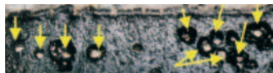
Fig. 3: Formation of bubbles after 2.5 years of weathering. Opposing contact area between joint sealant and concrete edge.
