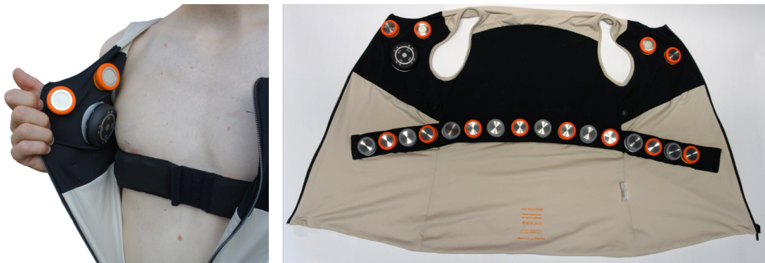
Figure 4.9 – Wearable EIT system integrated in a vest with the master sensor (black), the type V sensors (orange), and the type I sensors (grey).
