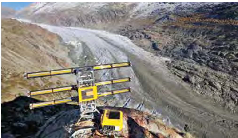
Ground-based radar and laser measurements monitor changes in the Moosfluh.
