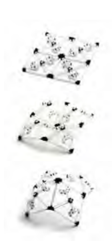
An object is printed flat and later converted into two further stable shapes.
