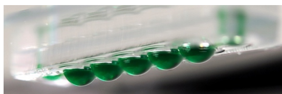
Figure 1 Photograph of a line of hanging drops filled with green food dye. As a result of surface energy minimization, all five hanging drops have the same radius and, therefore, comprise the same liquid volume.
