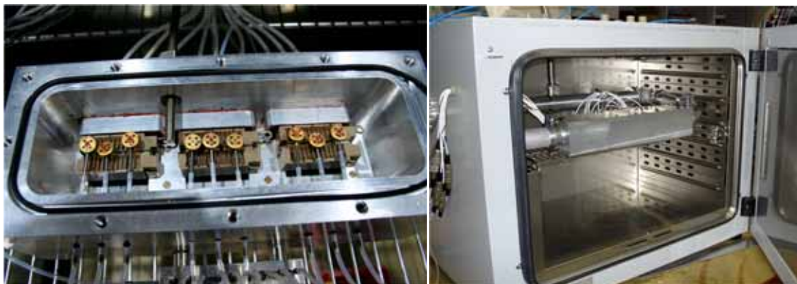
Fig. 2-8 High temperature sustainable pressure chamber (left), to be positioned within our laboratories sensor oven facility (right).
