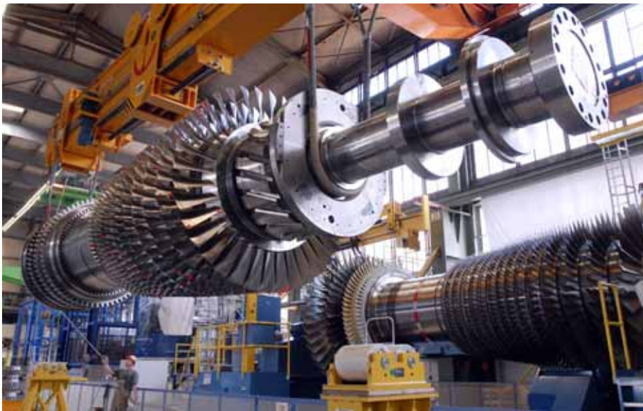
Fig. 1-2 Core part of Siemens 340 MW Gas Turbine SGT5-8000H (courtesy of Siemens).
