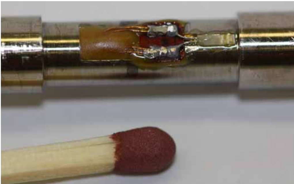
Fig. 3-8 Probe shaft temperature sensor installation on 6mm shaft, compared to a match for scale comparison.
