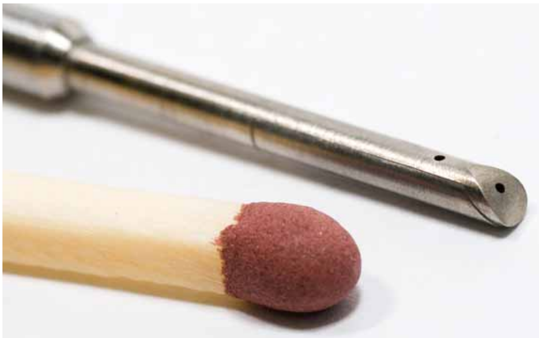
Fig. 5-7 Picture of standard FRAP probe compared to a match for scale comparison.
