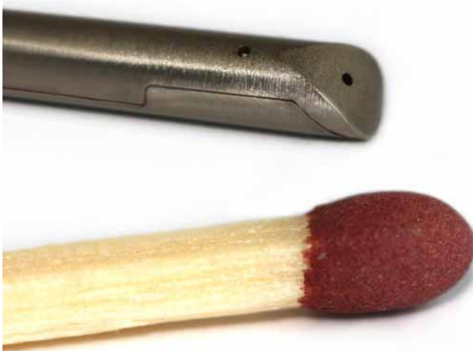
Fig. 3-1 Close -up view of FRAP-HT probe tip compared to a match for scale comparison.
