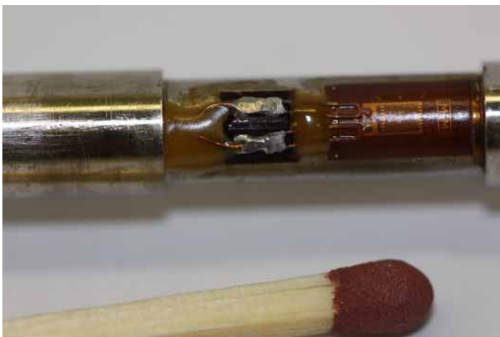
Fig. 3-7 Probe shaft strain gauge installation on 6mm shaft, compared to a match for scale comparison.
