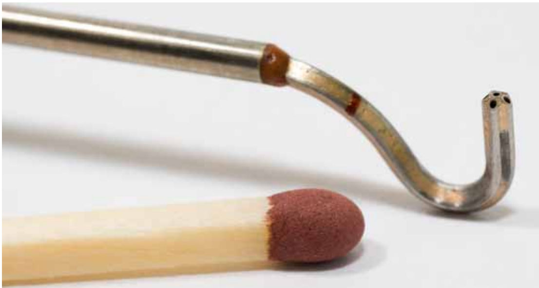
Fig. 5-3 Cobra-shaped 5-hole probe compared to a match for scale comparison.
