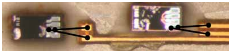
Fig. 2-13 Specimen of dummy sensors, connected via wire-bond (black lines) to the flexprint pads for bonding characteristic tests.
