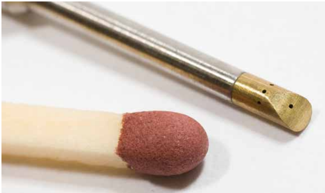
Fig. 5-1 Cylindrical 4-hole probe (FRAP shape) compared to a match for scale comparison.
