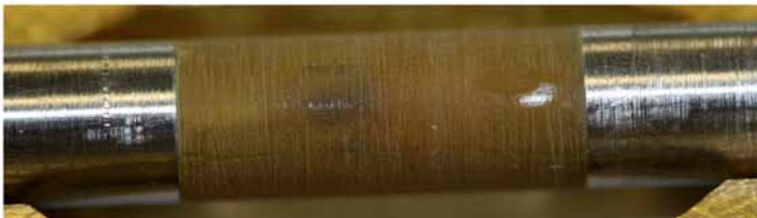
Fig. 3-9 Final view of covered slot on 6mm shaft, containing the strain gauge device and a PT100 temperature sensor.
