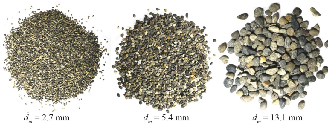
Figure 4.8 Uniform bed material with standard deviation of grain size distribution \sigma_g \approx 1.1
