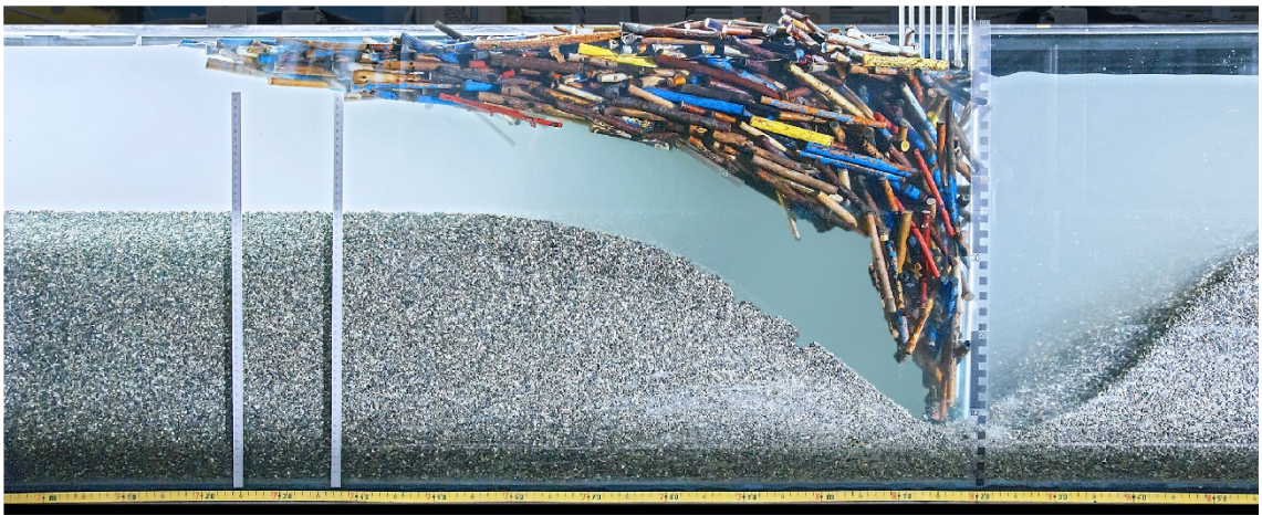
Model large wood accumulation at a retention rack with a movable bed
