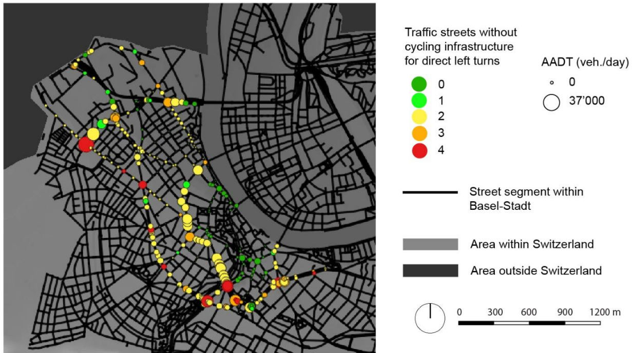
FIGURE 8 Number of traffic streets without cycling infrastructure for direct left turns, for each intersection in the case study area
