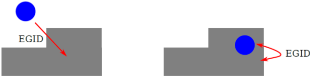
Figure C.15: Matching strategy with typographic error corrections for buildings with matching EGID. Red arrows indicate that EGIDs do not match. This relation is only valid if the mismatch of the EGIDs can be explained by a typographic error.
