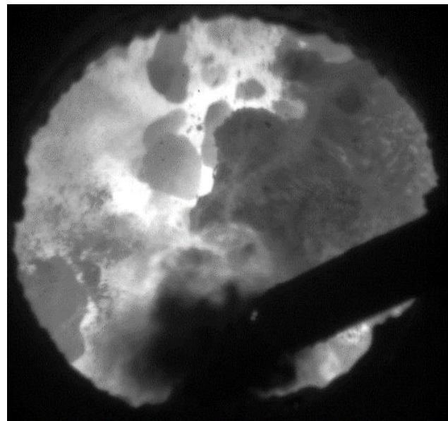
Fig. 4. Example of a partial raceway blockage.
