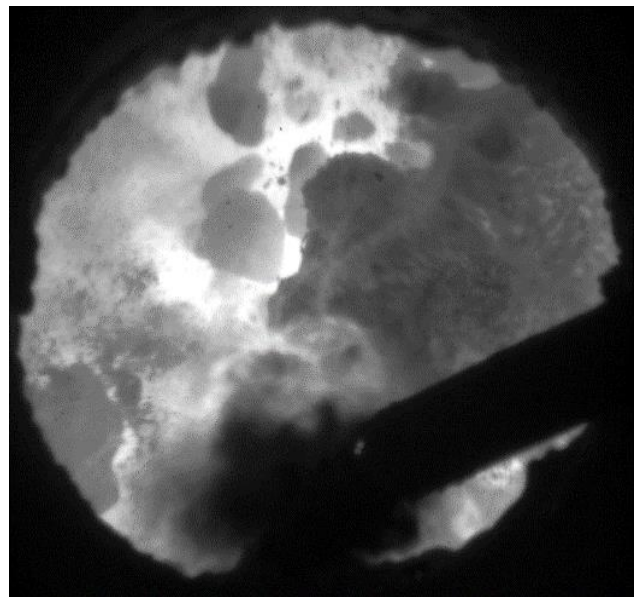
Fig. 4. Example of a partial raceway blockage.
