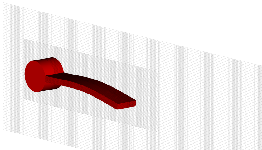
Figure 8.3: Snapshot of the computational domain, zoomed in on the cylinder-flag assembly.
