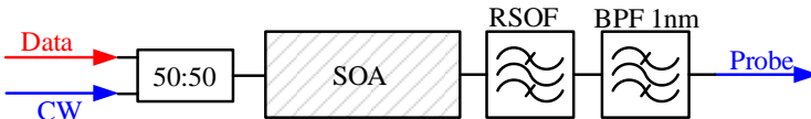
Fig. 5.20. Scheme of an all-optical wavelength converter utilizing a RSOF and BPF at \lambda_{CW} = 1536.3 nm, \lambda_D = 1530.0 nm .
