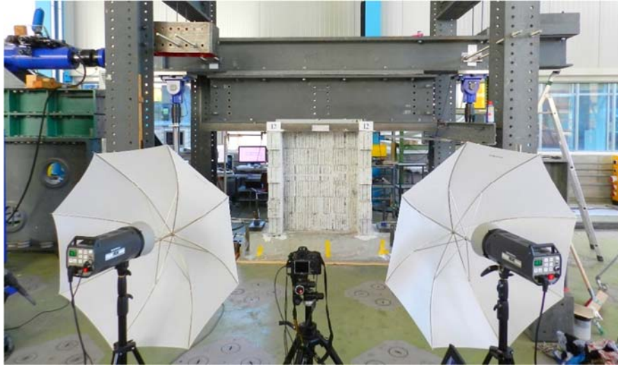
Figure 5-5. Implemented 2D-DIC measurement system [57]
