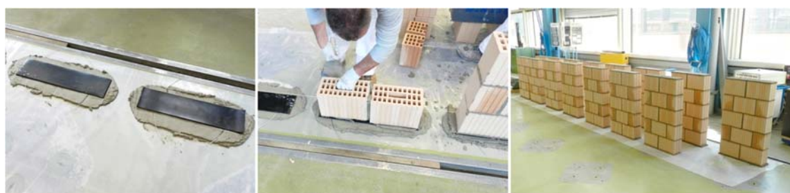
Figure 3-18. Construction and storage of the wallettes
