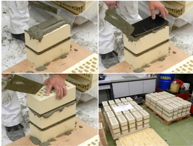
Figure 3-4. Construction and storage of the specimens
