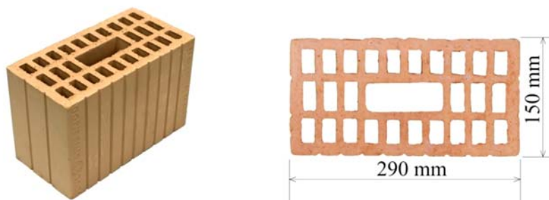
Figure 3-17. Swiss perforated clay block used for the construction of the wallettes
