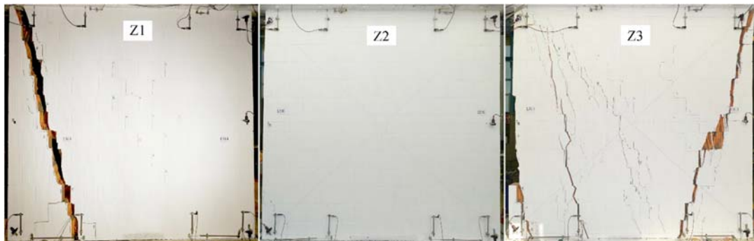
Figure 3-37. Final crack patterns of specimens Z1, Z2 and Z3 [40]
