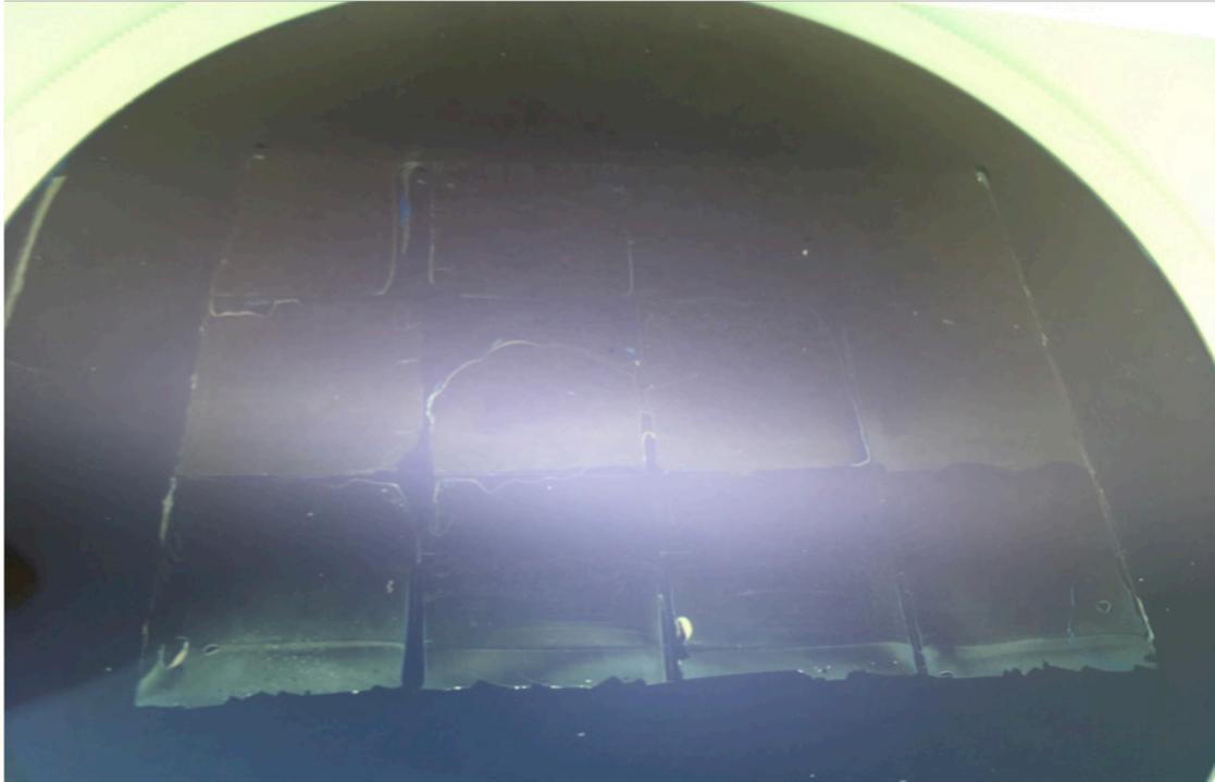
Figure 7.22: Photograph of the first sol-gel imprint on a 6" wafer with X-PDMS negative obtained from 12 nanoparticle-density gradients assembled on a 6" wafer.
