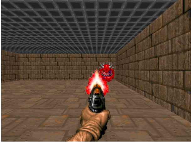
FIGURE 4.5: VizDoom simulated test environment. This image shows the simulated test environment used during algorithm development. The agent spawns in the center of a room and can perform one of only three possible actions: move left, move right or shoot. A stationary enemy is spawned at a random position along the back wall of the room. The challenge in this simple scenario involves aligning the player with the enemy and then shooting to eliminate the enemy. A positive reward is given for hitting the enemy, which also resets the episode. Negative rewards are given for wasting ammunition and time. We chose this scenario to evaluate initial algorithm performance, since it allowed algorithm testing at rates exceeding 500 frames per second.
