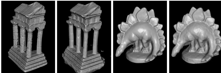
Figure 24: Ground truth surfaces and reconstructions for Temple Full and Dino Full of the Middlebury multiview stereo evaluation dataset [106].
