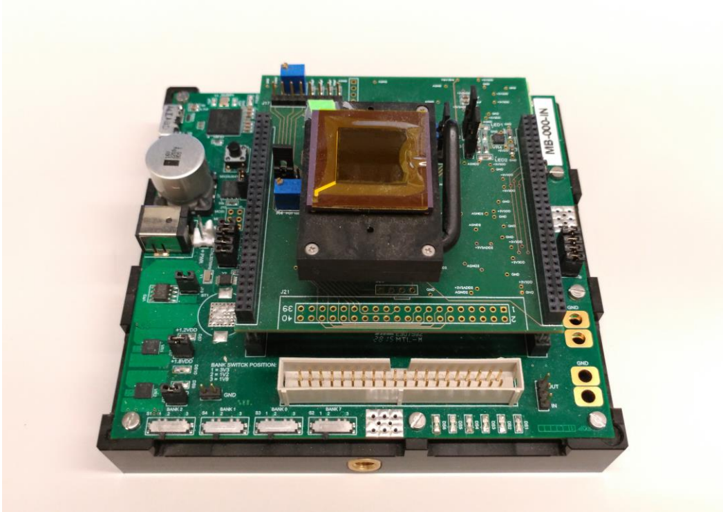
Figure 4.32 The PCB of the hardware system consisting of an FPGA LS an ASIC RS. The occupied area of the PCB is 127 \times 118 \text{ mm}^2 . The FPGA used is Lattice Semiconductor LFE3-70EA-FN484.
