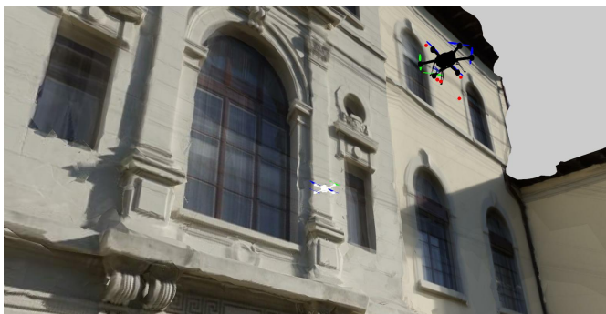
Fig. 3: UAV Master, in black with red marker, and the Slave, in white, in front of a large 3D Reconstructed facade
