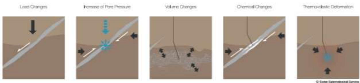
Figure 18: Schematic representation of the physical mechanisms that can induce earthquakes.
