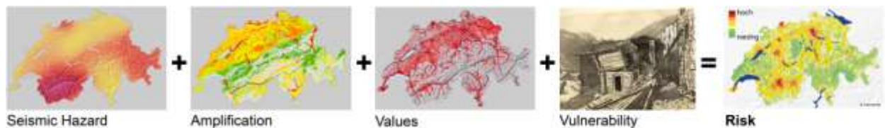
Figure 16: Seismic risk is a combination of seismic hazard, local soil conditions, exposed built environment and population, and vulnerability of the exposed structures.
