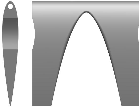
Figure 3.3. Side and top view of control flap 2. The flap has 80mm length (chord length) and 83mm width. Compared to the control flap 1, which has the same dimensions and the same airfoil (NACA0015), a triangular part of control flap 2 is cut out.
