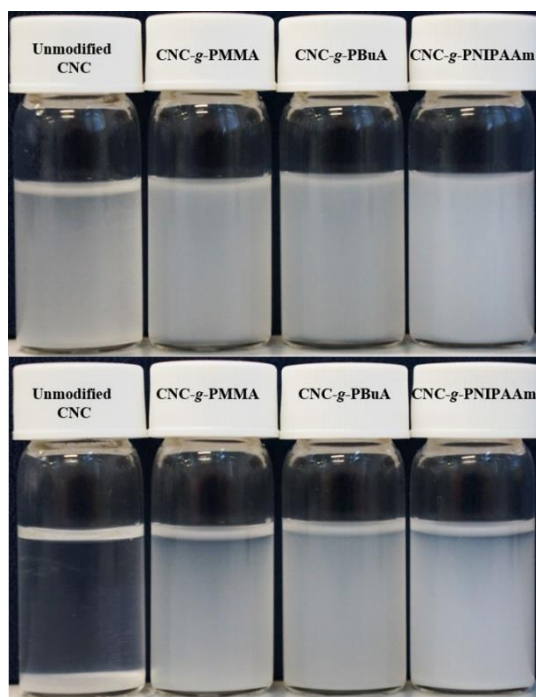
Figure 3.10 Dispersion test of unmodified and polymer grafted cellulose nanocrystals (0.5 wt%) in THF. The CNC- g -PHEA sample was not tested, since the homopolymer is insoluble in THF. Pictures recorded: immediately after stirring stopped (top), and four hours later (bottom).
