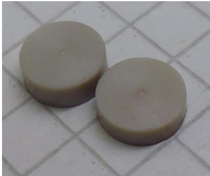
Figure 4.18: cylindrical samples of polyether-ether ketone cut out of spare heat transfer platforms for measurements of density, specific heat and thermal diffusivity and conductivity. Squares in the picture are 5mm in side.
