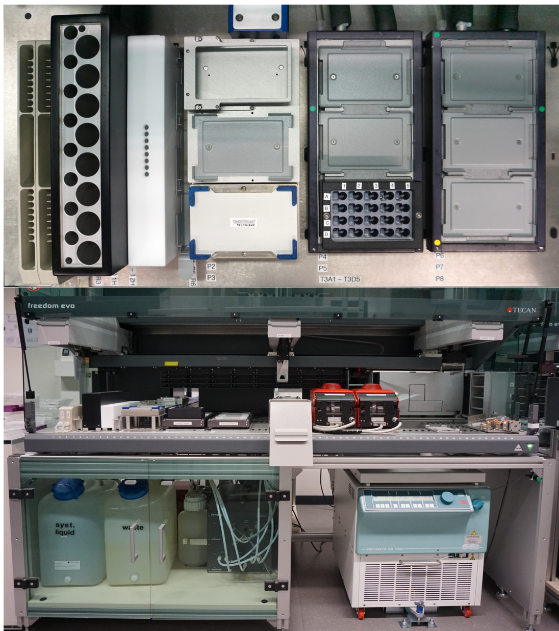
Figure 1.2: Tecan Evoware Freedom 200 . (Top) Top-view of the robot's pipetting area. From left-to-right: the washing station; tube holders; a large white trough; three 100 mL trough holders (empty); then 8 plate holders and an Eppendorf tube holder. The plate holder with blue edges is also a shaker. (Bottom) Front-view of the robot. From top-to-bottom: three robotic arms; the bench area with labware holders, two red thermocyclers, and a silver optical reader; system liquid supply, liquid waste containers, vacuum controller, and centrifuge.
