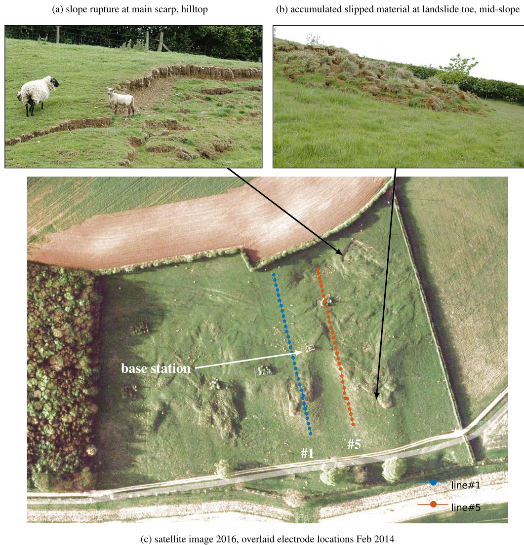
Figure 1. Slope failures at Hollin Hill; (a) rotational failures near the top of the slope above line#5, June 2015, (b) earth flow at the toe of a landslide where line#5 runs through mid-slope with electrodes throughout the slipped material, June 2015, (c) satellite image of the hillside (2016), showing four landslide ‘lobes’, five lines of 32 electrodes as of February 2014, and base station location. [(c) Satellite imagery ©2016 DigitalGlobe, Getmapping plc, Infoterra Ltd Bluesky.]
