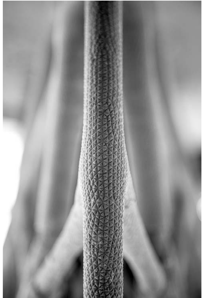
Figure 15: High resolution texture on the surface of the SkeleTHon. This texture maximizes the contact area with the waterproofing concrete skin. (DBT, ETH Zürich, 2017)
