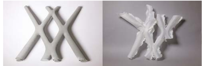
Figure 12: UHPFRC prototype (left) after the removal of the submillimetre formwork (right). (DBT, ETH Zürich, 2017)
