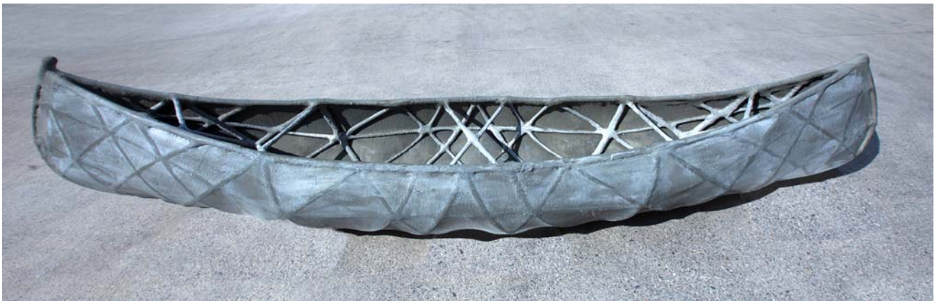
Figure 1: skeETHon, the four-meter-long canoe made entirely out of concrete. (DBT, ETH Zürich, 2017)
