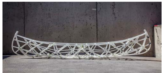
Figure 10: The 84 3D printed pieces assembled and ready for casting. (DBT, ETH Zürich, 2017)
