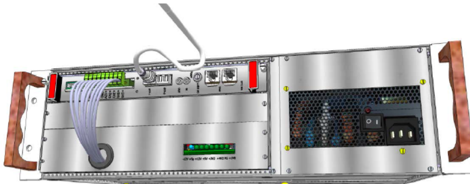
Figure 7.10: The 5 kg Mini-Crate to power the SRS Frontend. [146]
