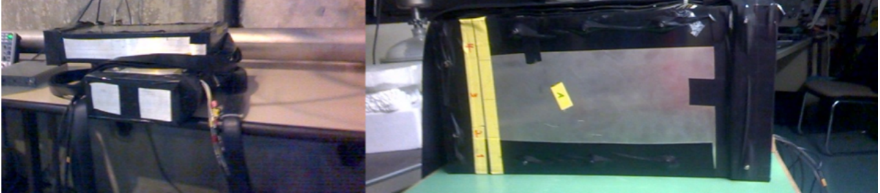
Figure 5.5: BGO modules in the aluminum box
