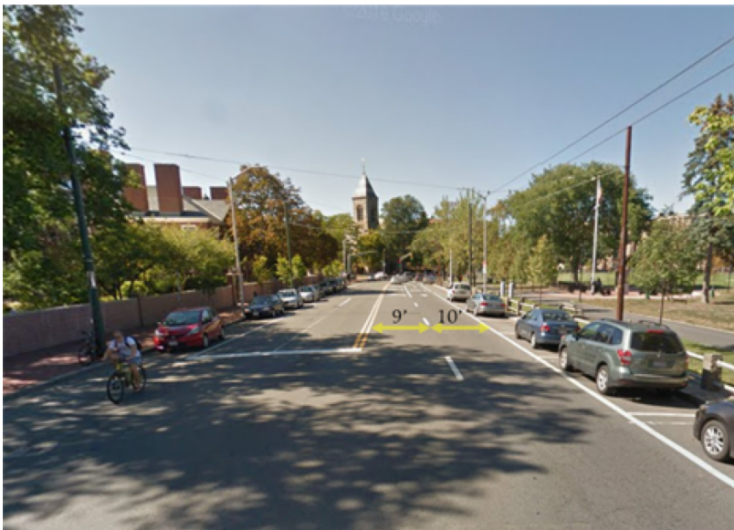
Figure 7.29: Example of 9' and 10' lanes in Cambridge, Massachusetts. Source: Adapted from Google Street View.
