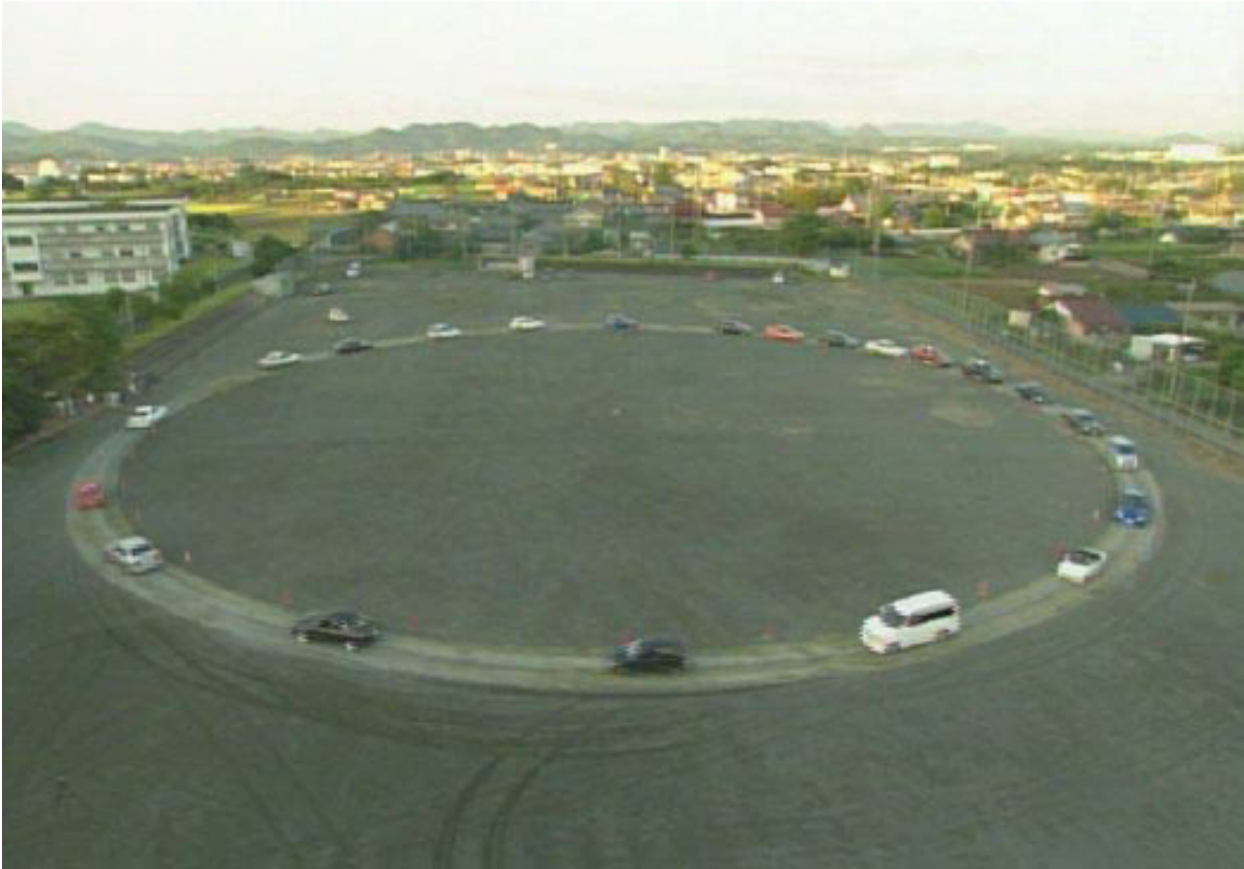
Figure 6.8: Shockwaves can form without bottlenecks. Source: (Sugiyama et al. 2008).
