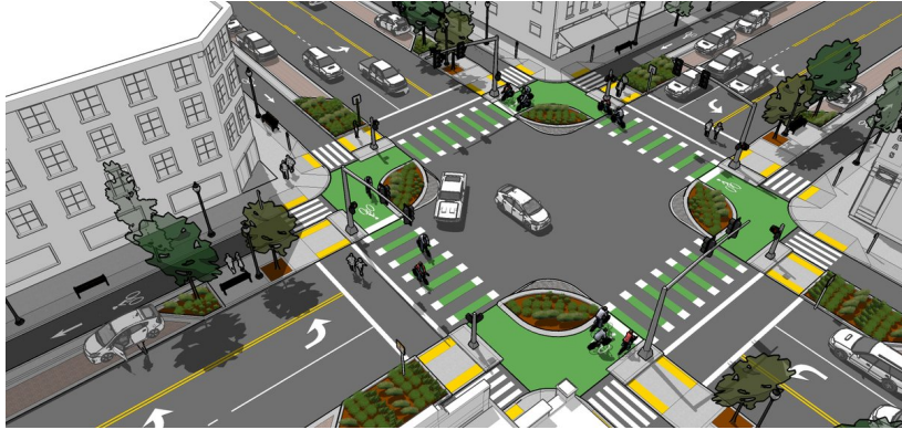
Figure 7.11: Protected bike intersection. Source: Alta Planning.
