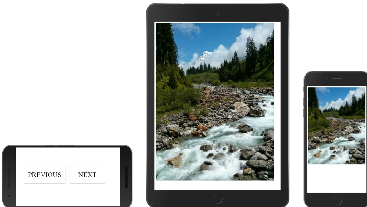
Figure 4.3: The controller example from Lst. 4.8 when loaded onto 3 devices. The first device has the controller role and shows buttons to navigate a gallery. The other two devices are viewers and display the selected image
