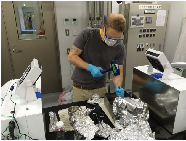
Figure 3. Example of sample homogenization within the KOACH benchtop laminar flow system at the Kochi Core Center. Photograph by Beth Orcutt.
