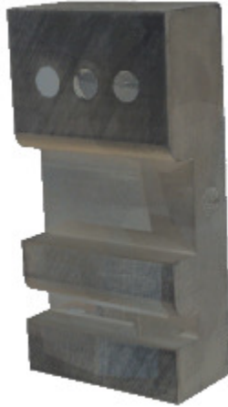
Figure 5.16: Optical scanning result of the test sample. This is the rendering of the mesh. Part of the texture is also recorded. The boundaries on the texture indicate the stitching boundaries. The visible surface of the sample is well represented. The mesh contains defects at the bottom of the trenches and the bottom of screw holes.
