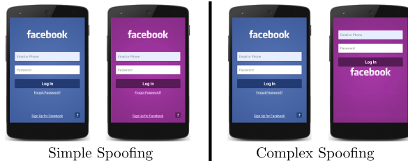
Figure 5.2: Examples of simple (changing background color) and more complex spoofing (repositioning elements).
