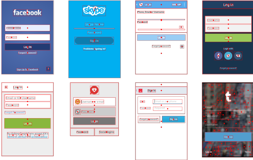
Figure 5.13: Decomposition examples. The login screen decomposition algorithm works well in practice. We outline in red the borders of detected elements, while the red diamond represent element centroids. Some login screens (tumblr, last screenshot) are visually complex and are inherently hard for our approach to analyze.
