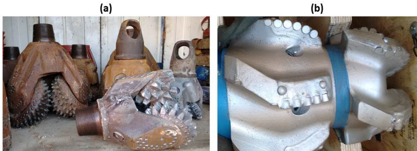
Figure 2.7: (a) Roller cone bits and (b) large-diameter PDC drill head, used at the geothermal site in Blanc-Mensil, France.
