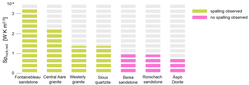
Figure 4.16: Results of the spallability validation. Experiment conducted at ambient conditions without external confining pressure. Rock-spallability calculated with Eq. 4.18
