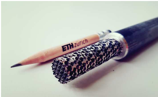
Figure 5.1: Laser sintered metal structure with inner diameter of 14 mm. The outer wall was partly removed for visualization purposes.
