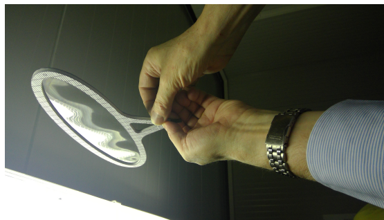
Figure 3.64.: The reflections on the target qualitatively show the wavy surface of the scintillator already before installation in COBRA. The scintillator was plane and showed a good mechanical stability before glueing to the Rohacell frame. For a final installation in MEG II the mounting technique of the target has to be improved in order to reach a better planarity which is not only beneficial for the profile reconstruction in a scintillation target but is of utmost importance for the MEG II analysis, independent of the stopping material used.
