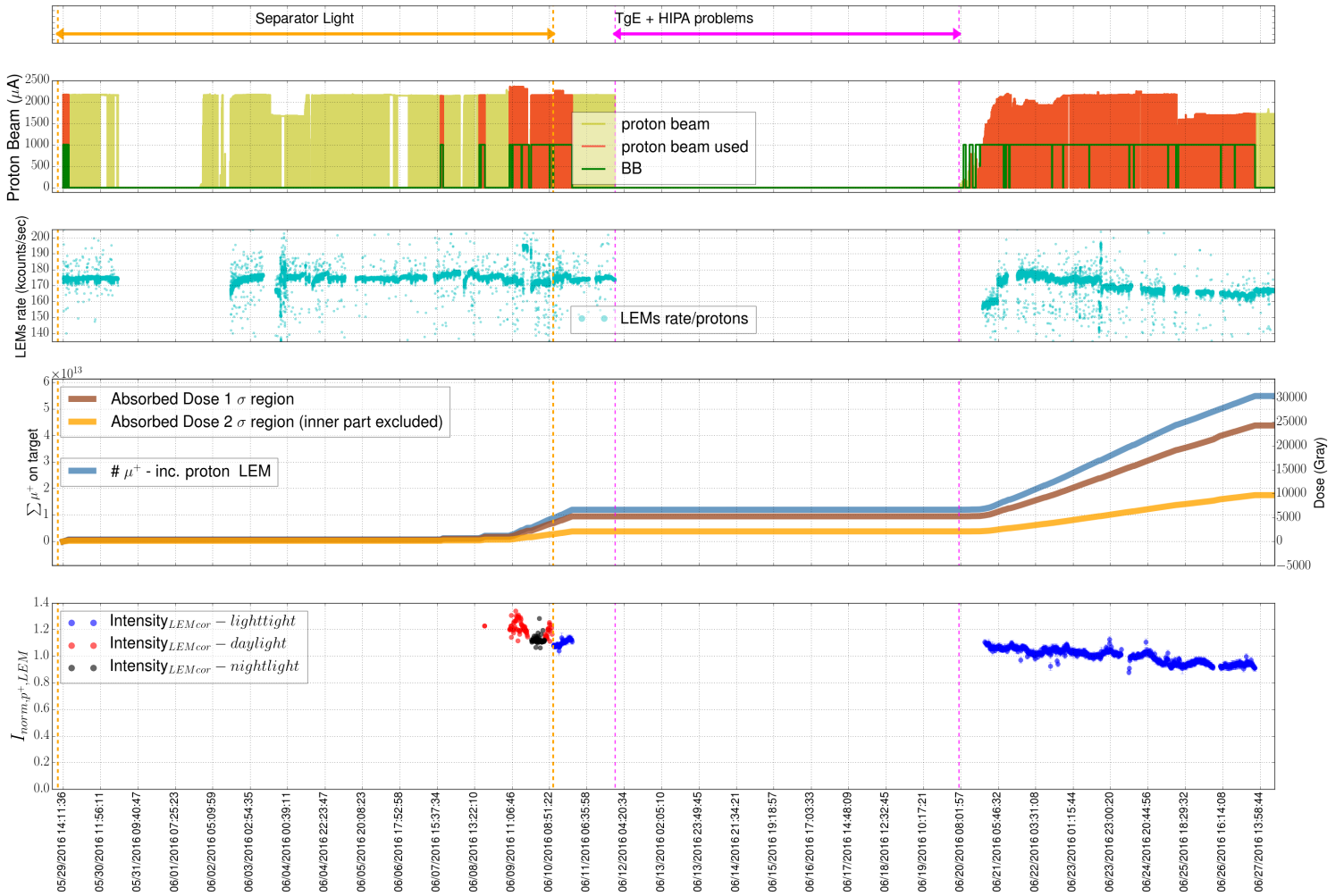
Figure 3.58.: Shows the relative scintillation target LY versus the accumulated number of muons on target and equivalent radiation dose, as well as the MHC_4 signal, BB information and the LEM rate.
