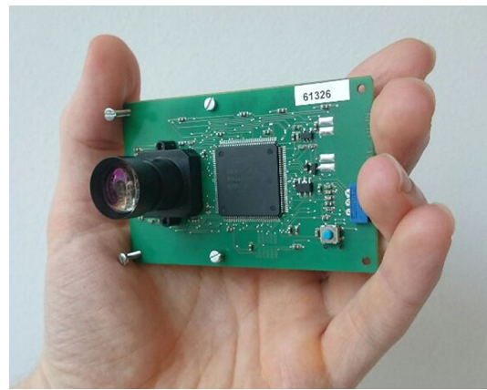
Fig. 1 The event camera “eDVS” produced by iniLabs ( https://inilabs.com/products/ )
