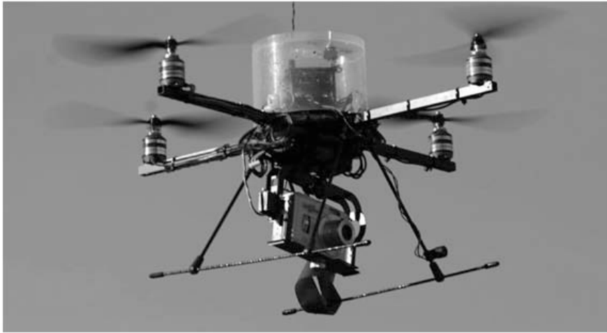
Figure 3-3: A Mikrokopter photo flight at Honggerberg, ETH Zurich (Eisenbeiss, et al., 2009b).
