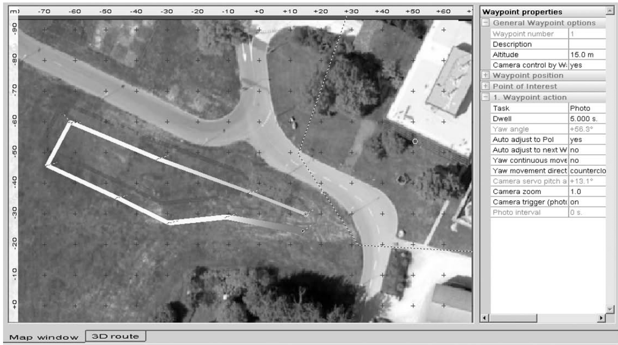
Figure 3-6: Screenshot of the waypoint editor of mdCockpit showing a plan of an autonomous flight at the campus ETH Hönggerberg.
