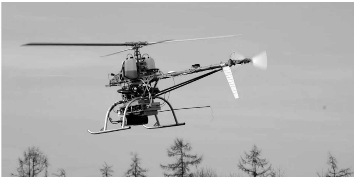
Figure 2-8: The scout B1-100 equipped with the Riegl airborne LiDAR scanner LMS-Q160.
