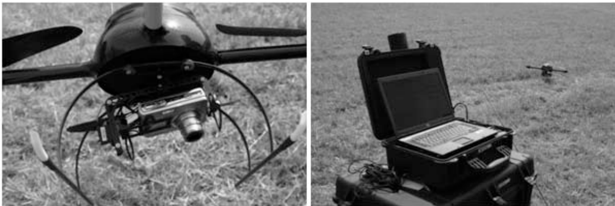
Figure 3-5: Left: A detail view of the system showing the adapted camera. Right: Ground Control Station.
