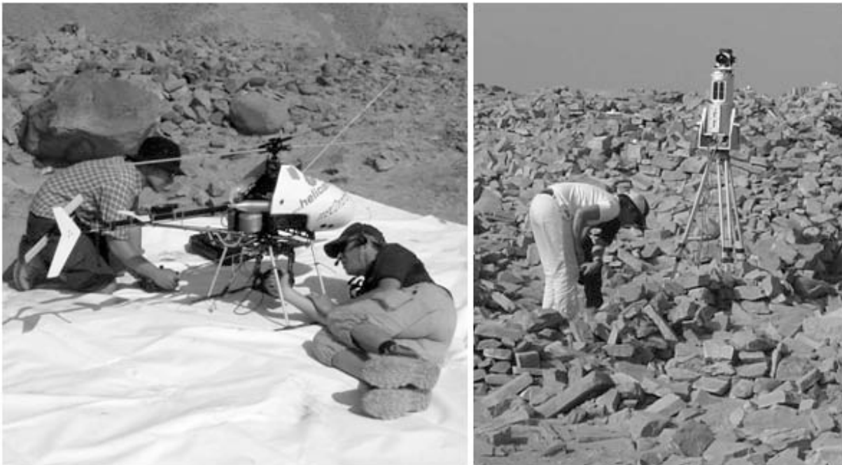
Figure 6-4: Left image shows the selected mini-UAV system, while the right image illustrates the chosen terrestrial laser scanner RIEGL LMS 420 at Pinchango.
