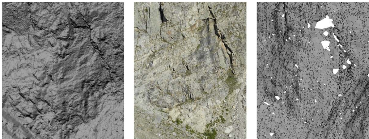
Figure 7-7: Left: Derived surface model from image matching, Middle: Zoom-in of an UAV-image, Right: Point cloud of Helicopter-based LiDAR projected on the derived surface model.
