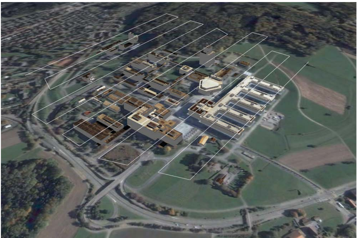
Figure 4-1: Flight plan for an UAV flight over Campus ETH Hönggerberg visualized in Google Earth (Source: Bare ground and DSM (Google Earth) and 3D Model of Campus Hönggerberg (IGP, ETH Zurich)).
