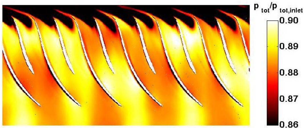
Figure 5.12.: Relative total pressure distribution for OL1.
