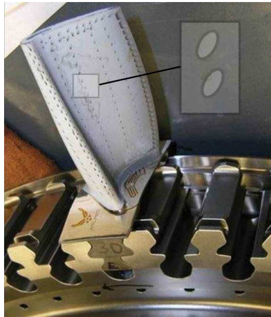
Figure 1.4: A film cooled blade from the high pressure turbine of a Pratt and Whitney F135 engine
