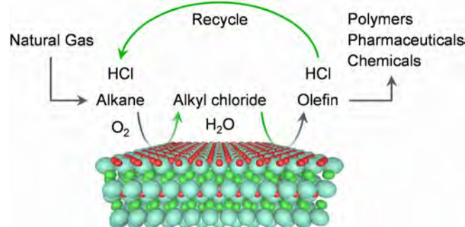
Figure 1. Closed-loop chlorine-mediated process for the one-step conversion of abundant light alkanes to valuable ethylene and propylene, which are the main building blocks of the chemical industry. An optimal catalytic material for this process should integrate the ability to functionalize the alkane into the corresponding alkyl chloride and to dehydrochlorinate the latter to yield an olefin, enabling the full recycle of the halogen source.
