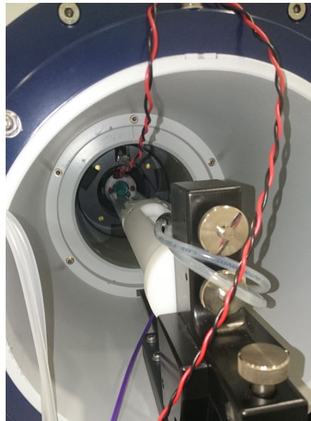
(c) PCB holder inserted in MRI bore with power cable (red and black) and optical fiber (purple) running out.
