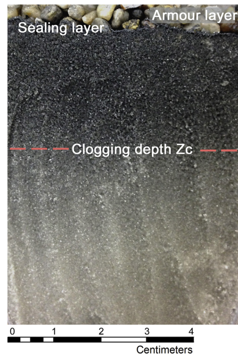
Fig. 1. Illustration of clogging depth, sealing and armour layer. Photographs from laboratory experiments with a profile with a decreasing number of retained particles with depth and a specific clogging depth Z_C .
