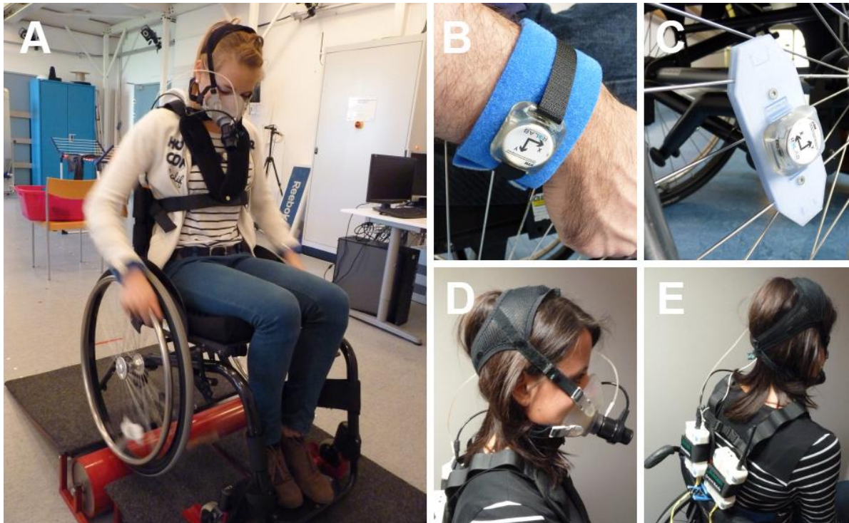
Figure 6-1: A: Examiner wearing the full experimental setup during the activity training on the wheelchair ergometer. One sensor module was attached at each wrist, one at the chest and one on the wheel of the wheelchair. B: Sensor worn at the wrist with the AlphaStrap Blue and Velcro Strap fixation. C: Wheel sensor with dedicated attachment. D: Oxycon mobile mouth piece. E: Back view of the Oxycon Mobile with sensor box and data exchange unit.
