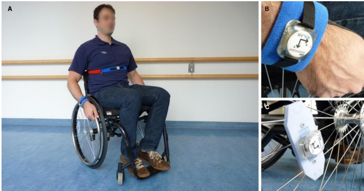
Figure 5-1: A: Attachment of the sensor modules to the subject. One module is attached at each wrist, and an additional module is attached at the chest. The fourth ReSense module is attached to the wheel of the wheelchair B: Module worn at the wrist with the AlphaStrap Blue and Velcro Straps fixation. C: Custom made fixation plate for the wheel module.
