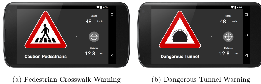
Figure 3: Two examples of the in-vehicle warning intervention shown to drivers approaching an accident hotspot
